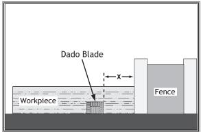
Figure 51. Illustration of a dado cut.
